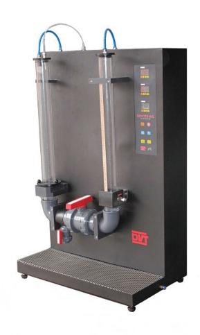
FOR MEASURING WATER PERMEABILITY OF GEOTEXTILE PRODUCTS
